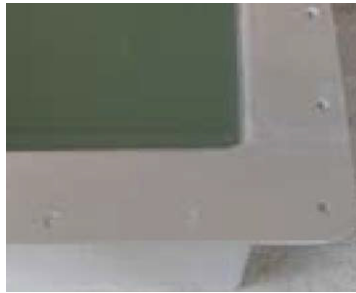
Ensure flanges are clean and free from grease, grit etc.
