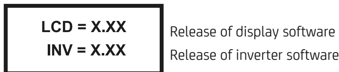
Figure 13.28: Display shown when first powering VASCO
