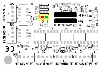
NOTE it is critical that J23 is reverted to the <u>normal</u> operating position (position 1) after diagnostics, to ensure correct Fire Sprinkler operation.
