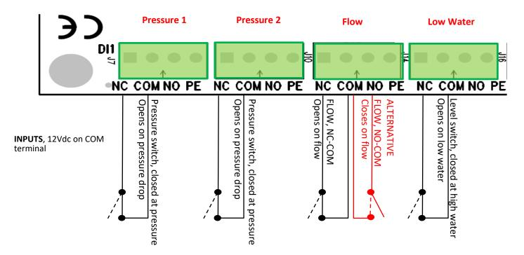
If a low water sensor is not required the input MUST be linked across to prevent alarms.
