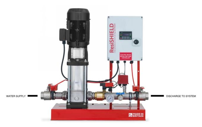
RV pump sets include a return loop to suction side from auto test drain, hence there is no dedicated outlet to drain required. However if the installer prefers to route the test outlet to drain or back to the tank, it is acceptable to blank the 1/2" return connection on suction pipe and re-route the pipework accordingly.
