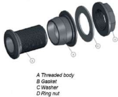
Fitting exploded view
